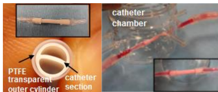
Figure 6.2. Thrombogenicity testing of catheter sections in a bioreactor under flow.
