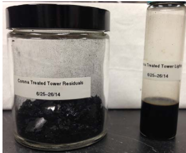
Figure 27: Corona and thermally treated test 6.25.14 carbon residue (left) and condensate (right)
