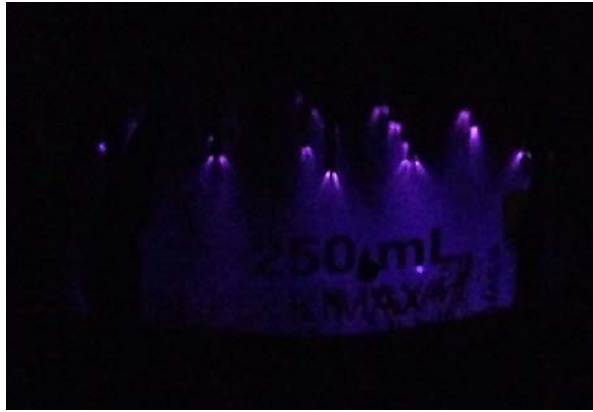
Figure 13: 19-point HV electrode over oil c with D_o=20 mm and D_p=15 mm at V=15 kV and I=0.188 mA, exposure time 1/15 sec.
