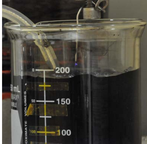
Figure 8: Single HV point over oil c with D_o=20 mm and D_p=10 mm
