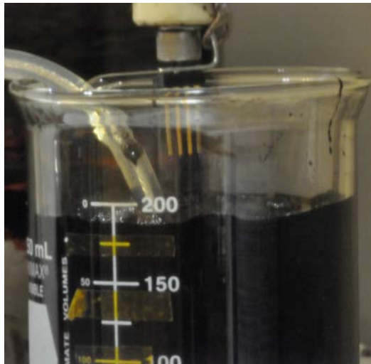
Figure 9: 4-point HV electrode configuration over oil c
