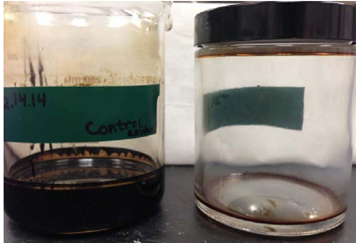
Figure 30: Residue (left) and condensate (right) for control test 2.14.14 at \dot{V}_{H2}=0.10 L/min and T_1 \neq T_3
