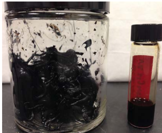
Figure 28: Corona treated test 6.4.14 corona residue (left) and condensate (right)
