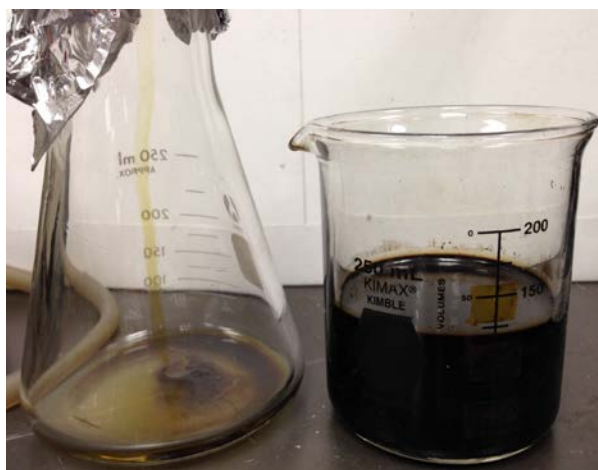
Figure 26: Condensate (left) and corona residue (right) produced from control test 7.15.14 at 600^\circ\text{F} \dot{V}_{H_2} = 0.40 L/min
