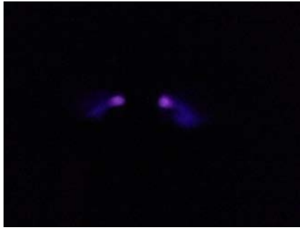
Figure 10: 4-point HV electrode with plasma discharge on outer two points, exposure time 1/15 sec.
