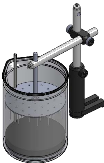
Figure 4: General configuration for corona treatment of heavy oil
