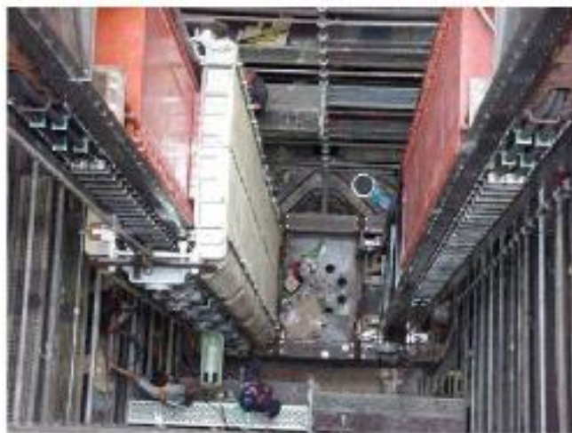
Fig. 5. The flat, double-sided linear PM machine built for the AWS (Copyright 2007 by IEEE)
