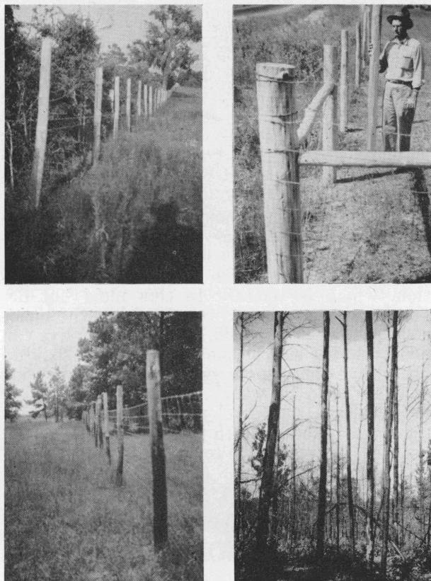
Figure 5. Dead pines like those pictured lower right are easiest of all woods to prepare and treat. The average-sized posts (4 inches in diameter) pictured upper right absorbed 1 to 2 gallons of borax-water. The posts pictured upper left were sealed at ground end with chromated zinc chloride. The posts pictured lower left were sealed with heavy oil at the ground ends. All of the sealed posts are still sound after 9 years in fences.
