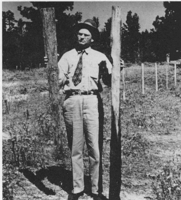
Figure 9. Split and sawed oak posts should be treated at the ground end with oil-type preservative as shown on the right. After a few years in the ground, only the top of the untreated post at the left remains.
