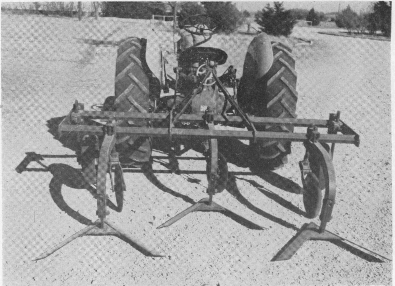
A sweep-type plow suitable for intensive cultivation.
