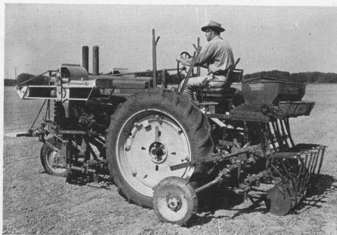
Experimental machine for applying various amounts of fertilizer and seeding simultaneously.
