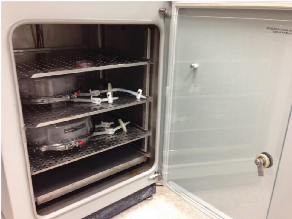
Figure 2-22. Hypoxic and normoxic setup for mammalian cell culture. A, Cells were placed in a closed chamber flushed with 2% oxygen, 5% carbon dioxide, and 93% nitrogen. B, The chamber was deposited in the regular cell culture incubator at 37°C to perform hypoxic cell culture. For regular cell culture (normoxic), cells were placed directly in the incubator as shown (Top shelf).
