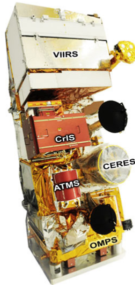
Figure 1.7: SNPP spacecraft and instruments (SSEC University of Wisconsin-Madison, 2012)
