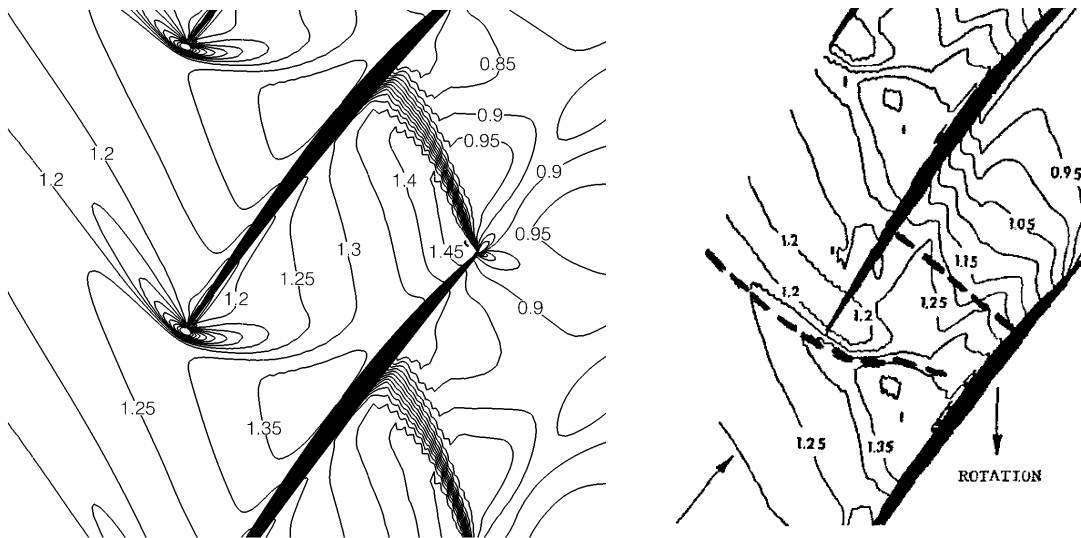
Figure VI.8: Predicted (left) and measured [Pierzga & Wood, 1985] (right) relative Mach number contours at maximum flow, and at 70% span.
