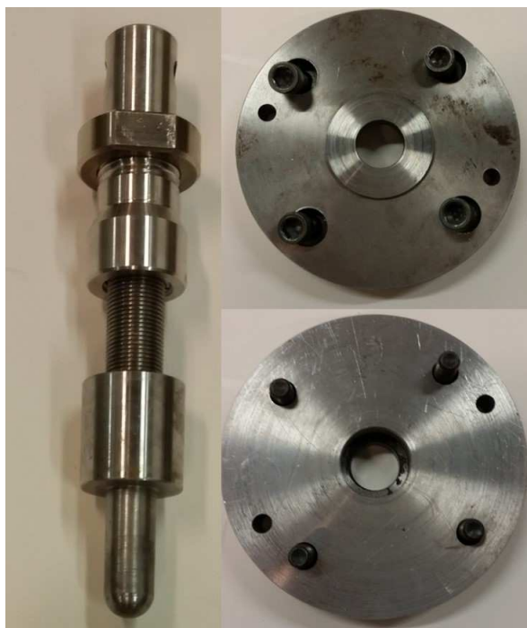
Figure 24: Geometry of the punch setup used in this study. The figure on the left shows the punch and to the right are the geometry of the die in which the plate was tested.
