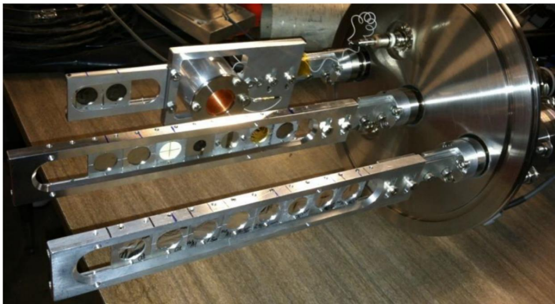
Figure 2.1. Target ladder assembly used in the experimental work. The first ladder (nearest to the bottom of the figure) held the Al degraders to vary the beam energy. The middle ladder held the various targets for calibrations and for the reactions studied in this work. The last ladder held the TC FC and the two ^{13}\text{C} charge equilibration foils.
