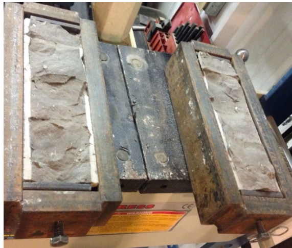
Fig. 6: Created Fracture Surface.
