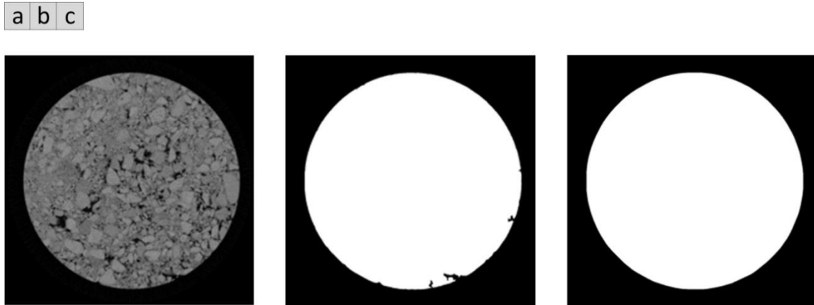
FIGURE 9 (a) Raw x-ray CT image. (b) Shrinkwrapped image. (c) Convex hull image.
