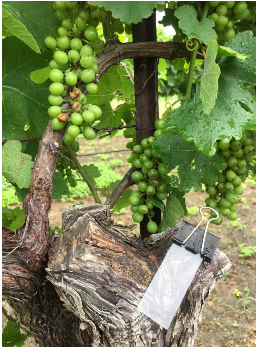
Figure 2 Glass microscope slide coated in petroleum jelly and attached to vine for the purpose of monitoring spore dispersal. Traps were collected and replaced once every 12 to 18 days over a period of six months.
