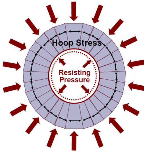
Fig. 1 - Representation of hoop stress with internal resisting pressure caused by hydraulic forces.
