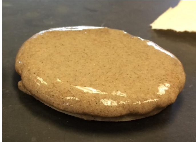
Fig. 12 - Base case after test 4, cake thickness 5.87mm.
