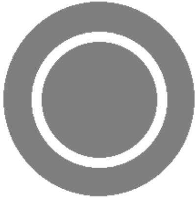
Figure 2: Schematic view of the face of the capacitive sensor. The grey portions are copper while the white is epoxy (not to scale)
