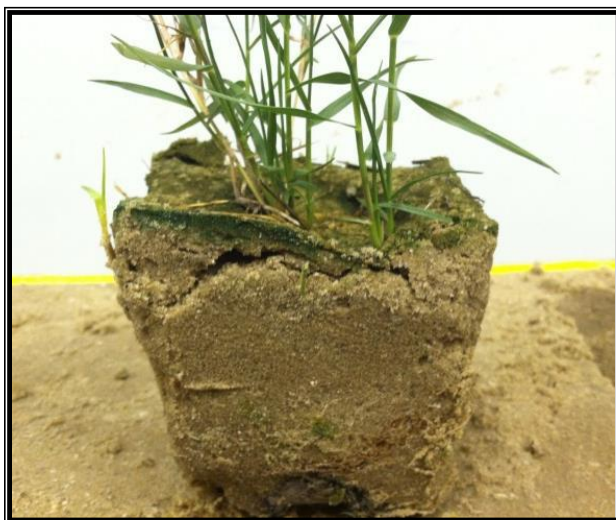
FIGURE 8: Sporobolus Virginicus . The native dune grass used for this experiment. Different increments of growth are transplanted into the swash zone of the wave flume (Figlus 4).
