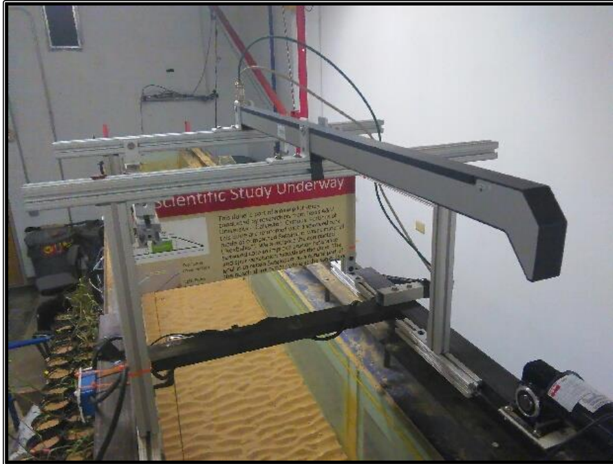
FIGURE 6: Laser Profiler. This figure shows the laser profiler mounted onto a moveable cart atop the MBWF.
