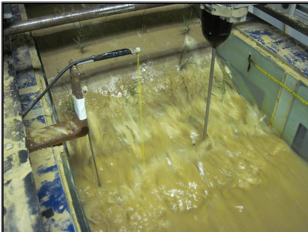
FIGURE 14: Vectrino Sensor Recording Swash Velocity.
