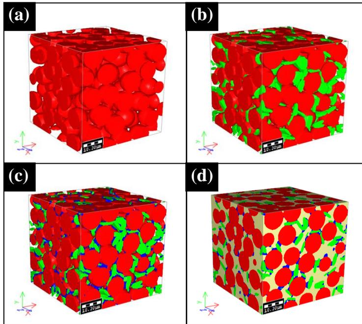
**Figure 3.** Electrode build process, as shown proceeding from left to right, then down. (a): Electrode is filled with active material particles (b): Conductive additives are added to the electrode (c): Binder is added between the active material and conductive additive particles (d): Remaining space is filled with an electrolyte.
