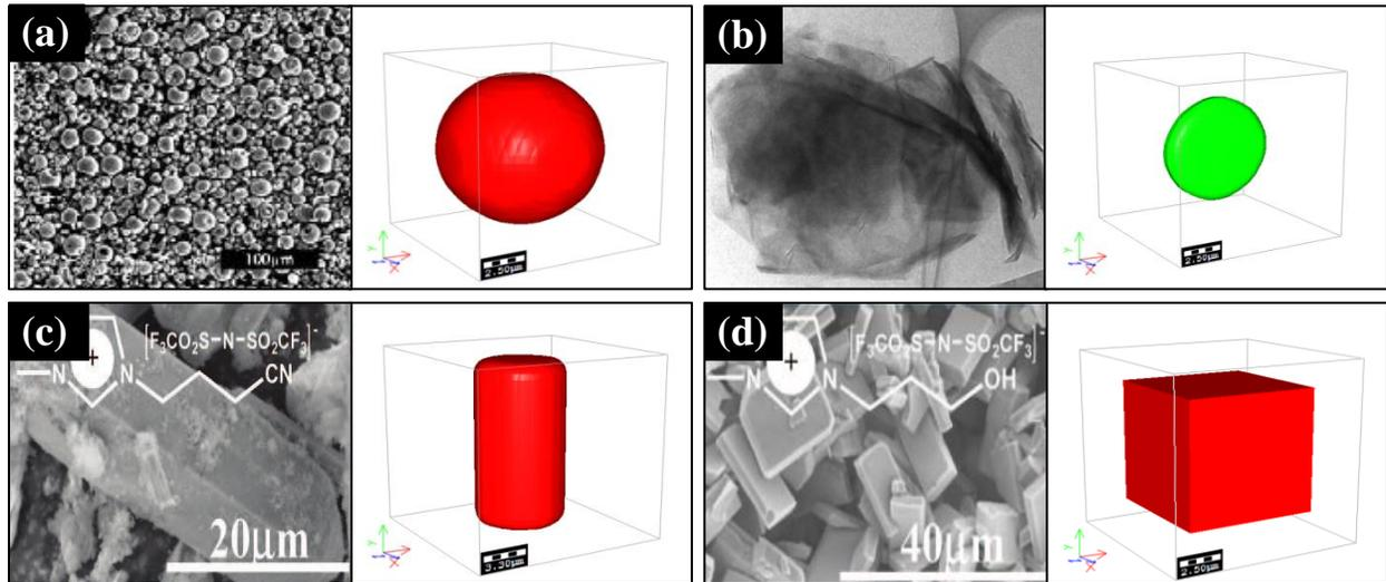
**Figure 2.** Stochastic modeling geometries for electrode constituents. (a): Spherical active material particles and stochastic representation [10]. (b): Graphite particle and stochastic representation [14]. (c): Cylindrical active material particle and stochastic representation [15]. (d): Cubic active material particle and stochastic representation [15].
