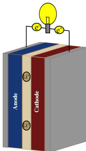
**Figure 1.** Typical sandwich-type lithium ion battery configuration.
