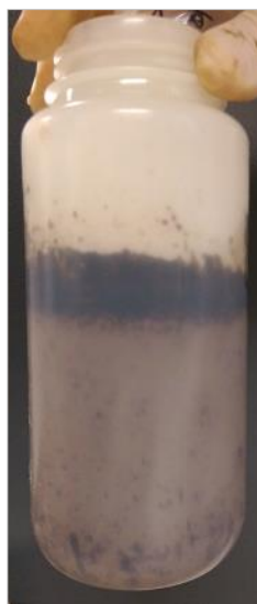
Figure A-3 – Picture showing the two phase separation of produced fluids in bottles
