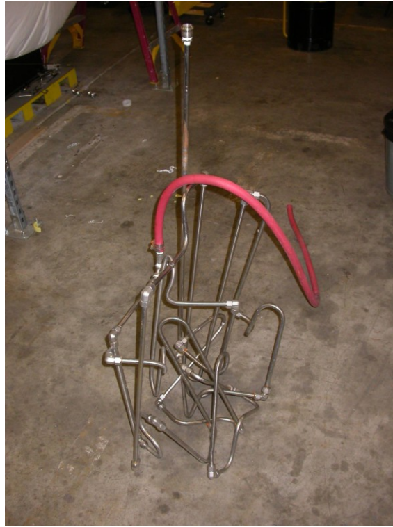
Figure 34: Heat Exchanger Tubing
