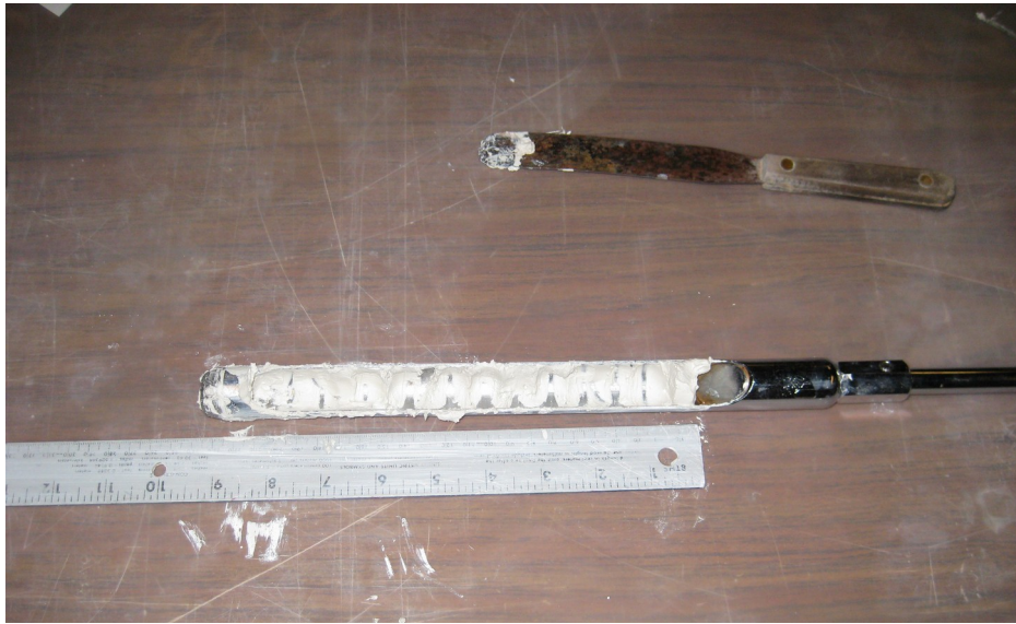
Fig. 4.22. Water content sampler used at T-bar locations
