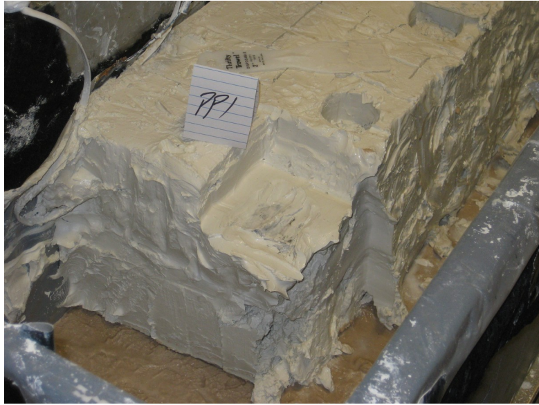
Fig. 4.21. Pore pressure excavation technique
