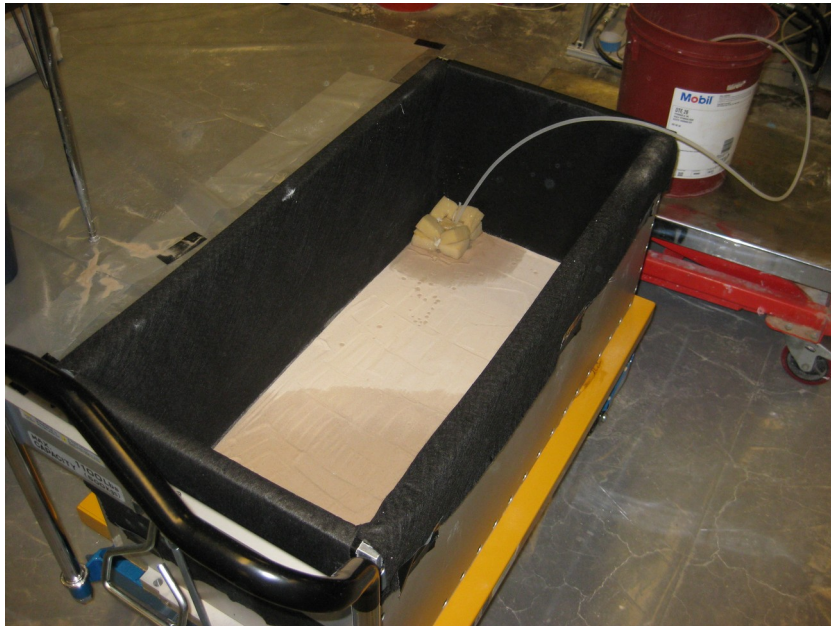
Fig. 4.12. Sand saturation processes
