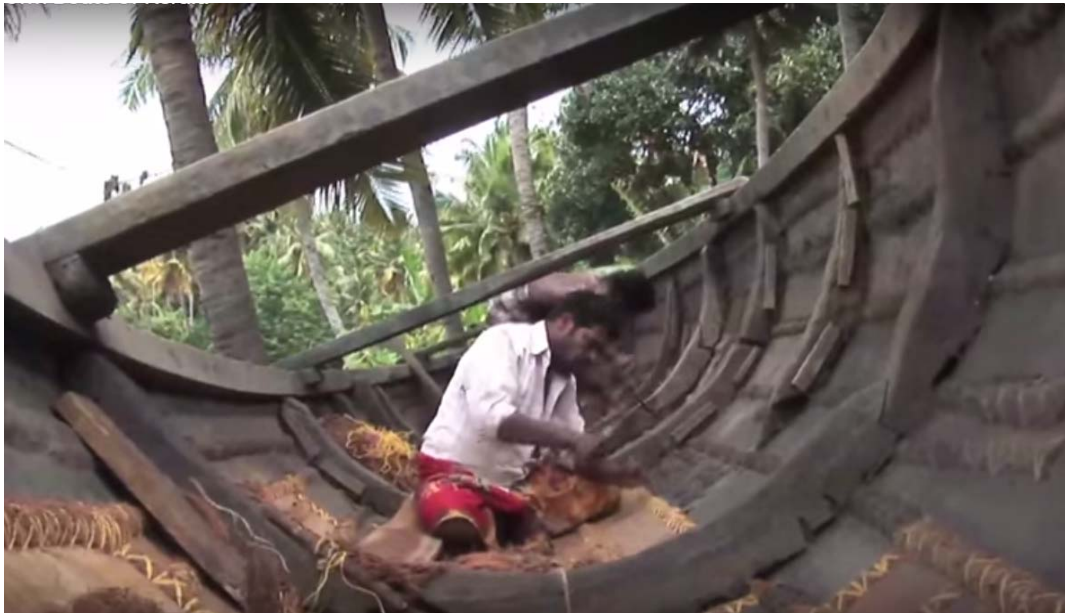
Figure 6.4: Lacers of the Kerala canoes in an angled position (Pomey 2012).
