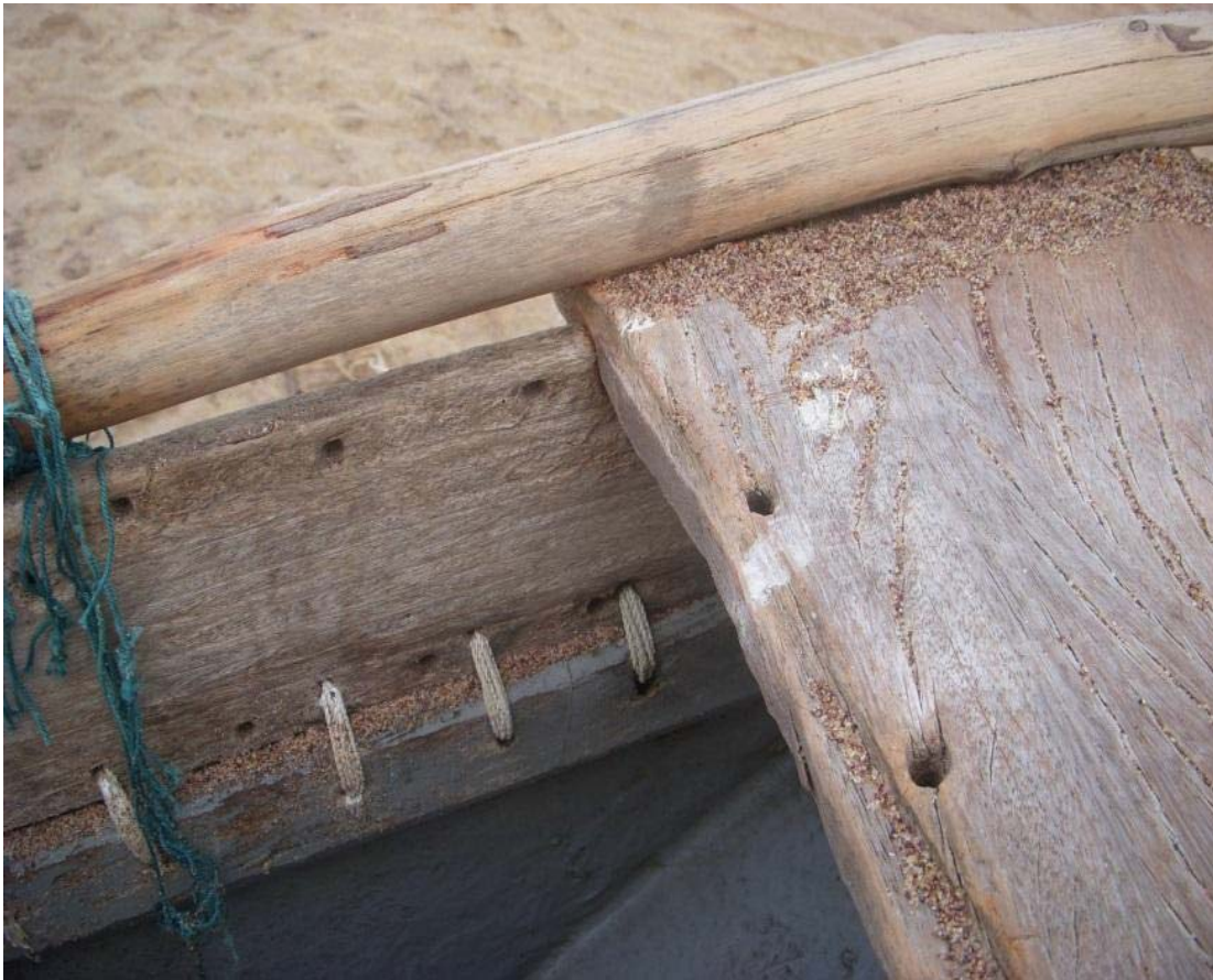
Figure 6.10: Reused laced washstrake as the stern bench of a laced oruwa of Sri Lanka. (Photo by author.)
