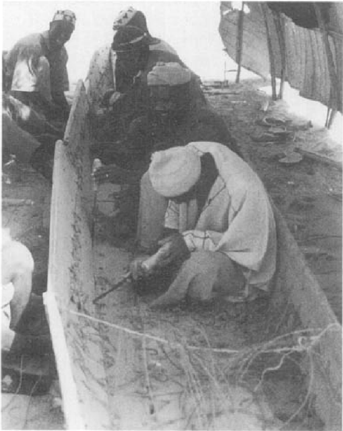
Figure 5.11: Builders of a laced boat in Gao, Mali work in tandem to repair the lacing (Insoll 1993, fig. 5).
