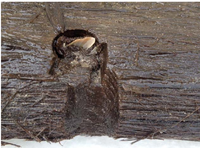
Figure 5.20: The external face of hull planking fragment 8 of the Venice Lido III timber assemblage showing two channels cut in opposite directions (photo by author).
