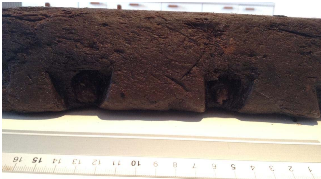
Figure 5.4: Edge cavities of hull planking fragment 1 of the Venice Lido III timber assemblage (photo by author).
