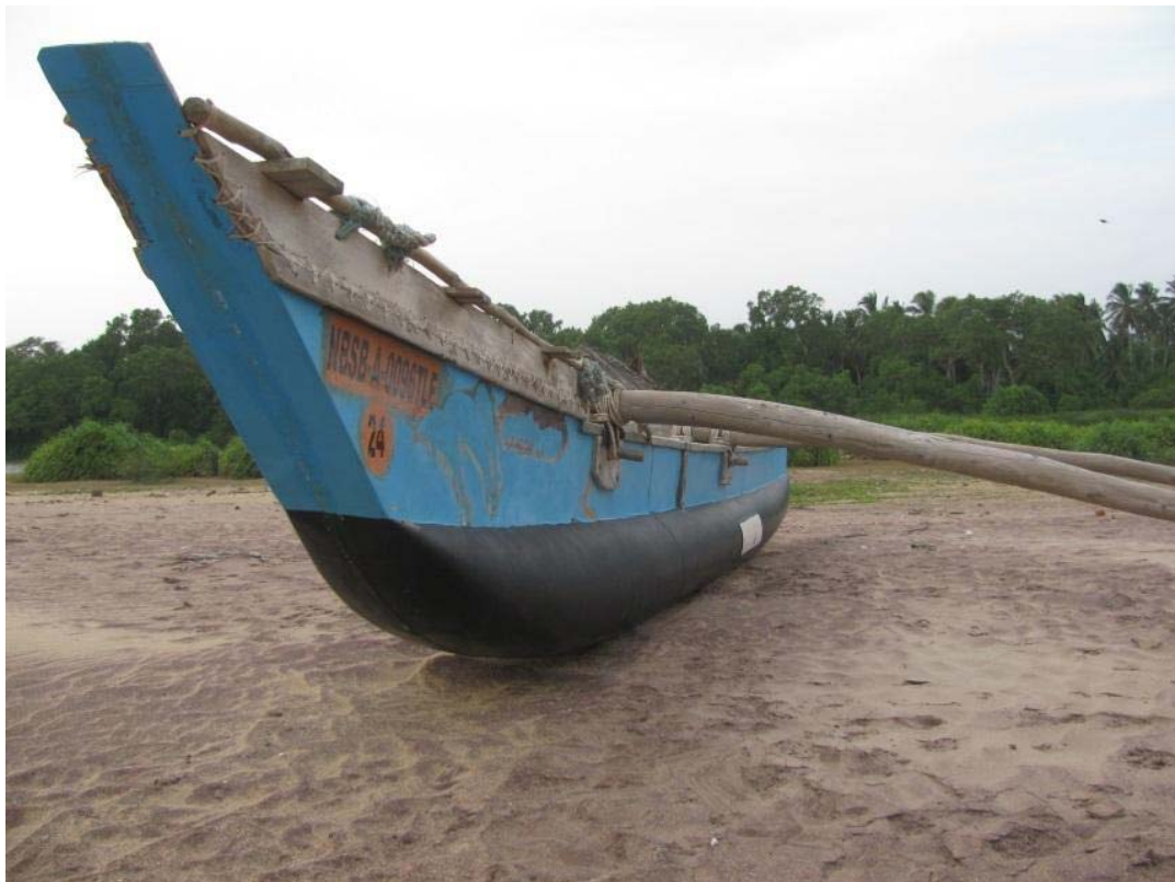
Figure 6.1: A laced oruwa of Sri Lanka with a fiberglass hull and wooden washstrake. (Photo by author.)
