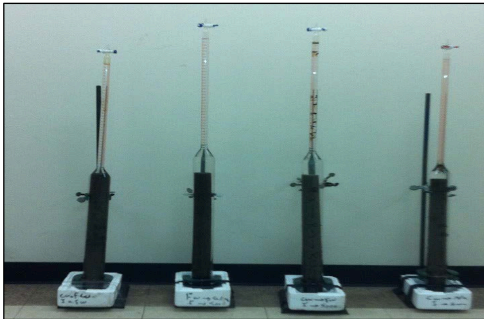
Figure 3 —Amott wettability cell for 1.5 in. diameter and 20 in. length cores for Bandera sandstone (R-1, R-2, R-3 and R-4) at the beginning of the test.
