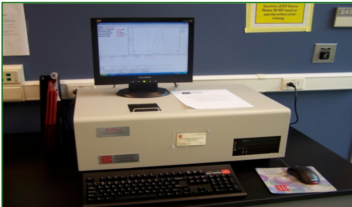
Figure 4—A photo of the ZetaPals setup used to measure the zeta potential.
