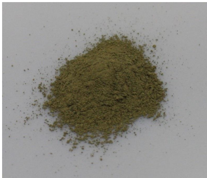
Figure 2.1: Synthesized BZF10 powder under 12 hours heat-treatment at 1600°C.
