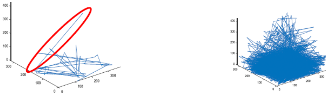
Figure 62: (a) The Least DTOF to the Top XY Plane for the Bottom XY Plane Seed Node Simulation, (b) The Maximum DTOF Path to the Top XY Plane Visualization for Bottom XY Plane Seed Node Simulation in Carbonate Pore Network
