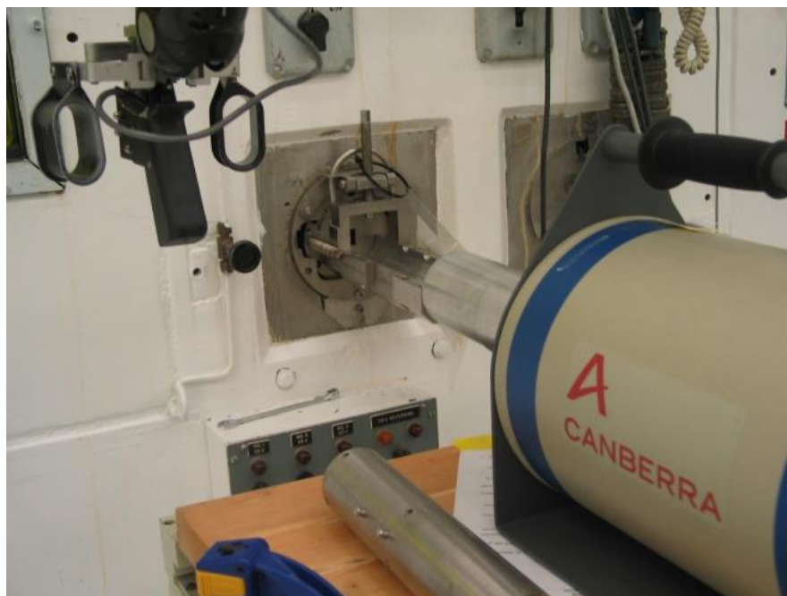
Figure 3.3. HPGe detector SNF photon measurement through the hot cell wall using the stainless steel collimator
