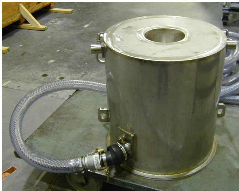
Figure 2.6. Fugen detector built for underwater measurements of Fugen fuel
