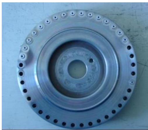
Figure III.6: The target wheel used for AMS measurements with aluminum cathode targets [64].
