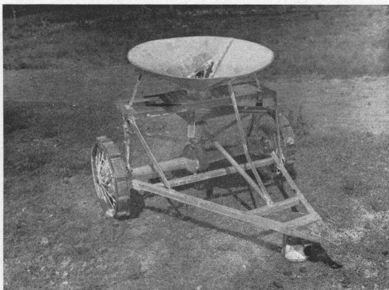
The auto-rear-end type of fertilizer distributor. Commercial machines of this type are now available. See description No. 3 on page 15.
