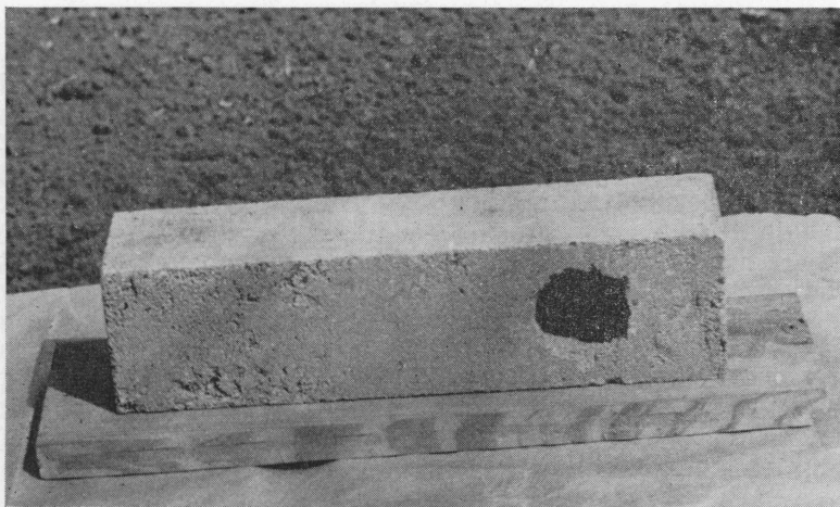
This tile, which was made about 3 hours before, is still on the pallet, and a hole has just been cut out in one side.
