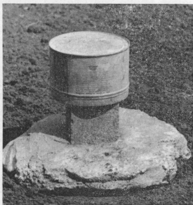
This tile, which was made about 3 hours before, is still on the pallet, and a hole has just been cut out in one side.
