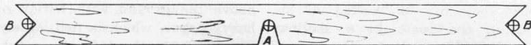
Figure 2. Planting Board. A, Stake in notch at center of board where tree is to be planted. B and B', Stakes in notches at ends of board to hold it in place. The stake A is removed when the hole is dug. When the tree is to be planted the board is replaced between stakes B and B' and the tree trunk is held in the central notch until the hole is filled with soil.
