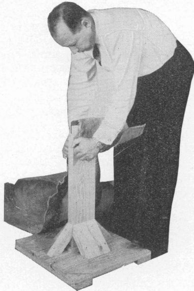
From time to time the directions call for "working" the leather until pliable. Above is shown a piece of equipment which may be used for this purpose, or a stout post or stake firmly fixed in the ground may also be useful.
