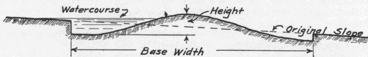
FIG. 3.—Cross section of a terrace before banks are plowed in, showing how dimensions are taken.
