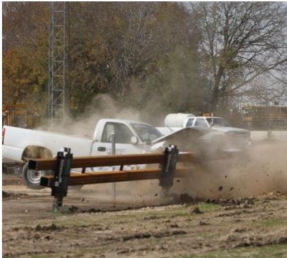
(c) Test and Simulation set-up at 0.5 seconds
