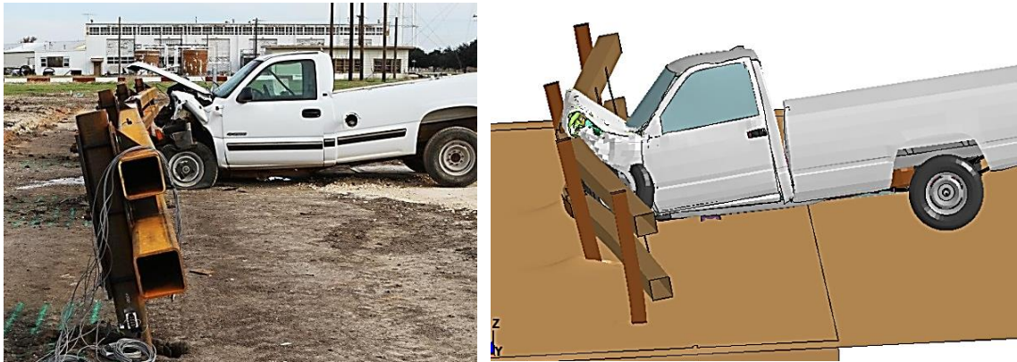
Figure 4-20: Numerical simulation of the impact test on a group of 4 piles
