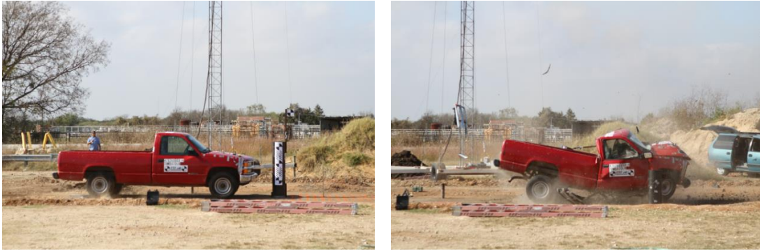
Figure 3-6: The pickup truck impact test PU60 (Mirdamadi, 2014)
