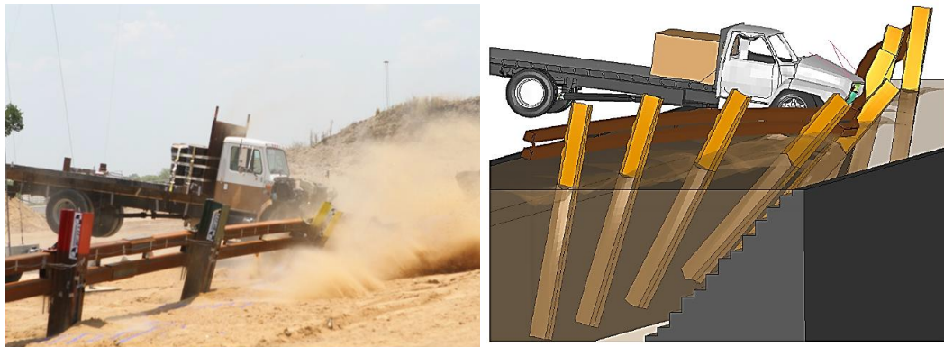
Figure 4-10: Numerical simulation of the impact test on a group of piles
