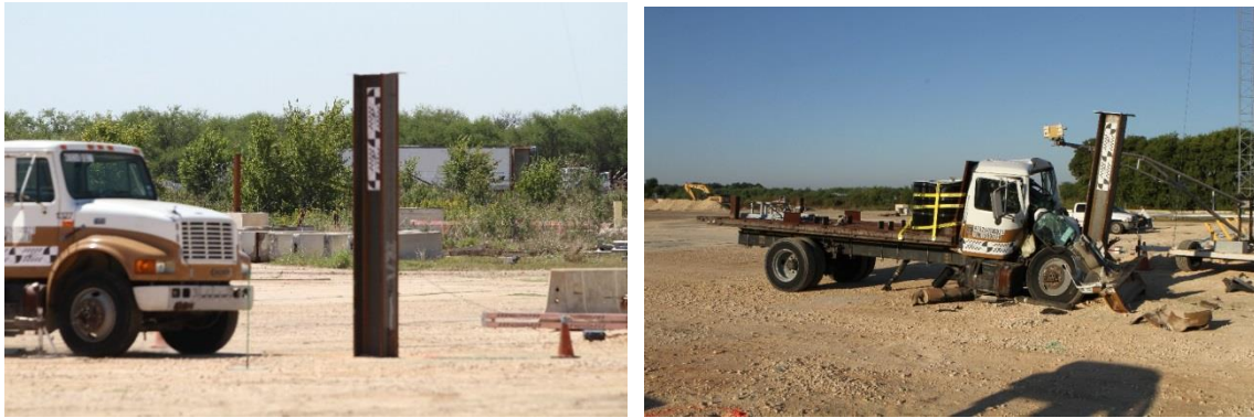
Figure 3-4: The test vehicle and the pile before and after the crash test (Mirdamadi, 2014)
