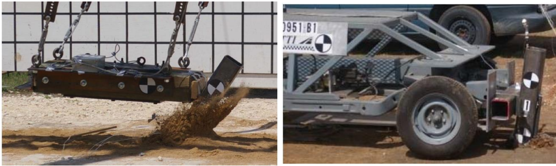
Figure 3-2: A Pendulum test on a single pile in loose sand (left); A bogie test on a single pile in stiff clay (right)
