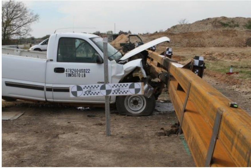
Figure 3-46: Vehicle and barrier after the impact on the group of piles system
