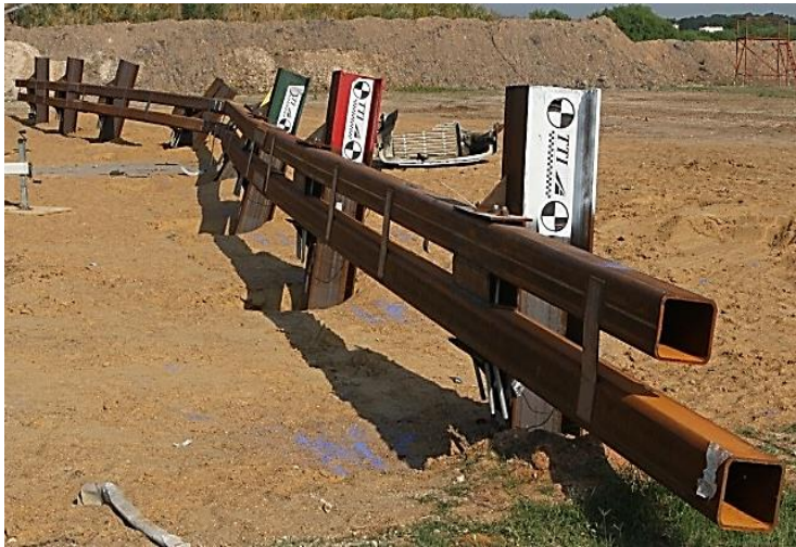
Figure 3-14: The group pile after the crash test M50
