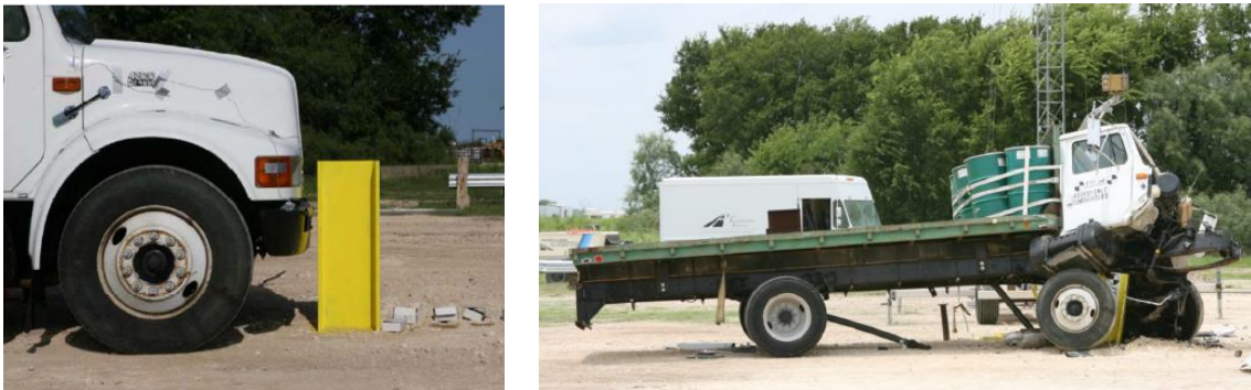
Figure 3-3: The test vehicle and the pile before and after the crash test (Alberson et al. 2007)
