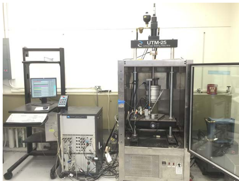
Figure 3.2 Configuration of Repeated Load Permanent Deformation Test
