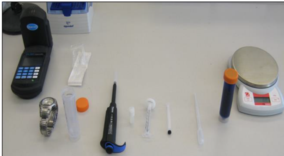
Figure 4.1 Test Devices for Methylene Blue Test
