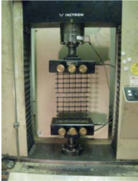
Figure 6.6 Direct Tension Test for Determining Sheet Modulus of Geogrid
