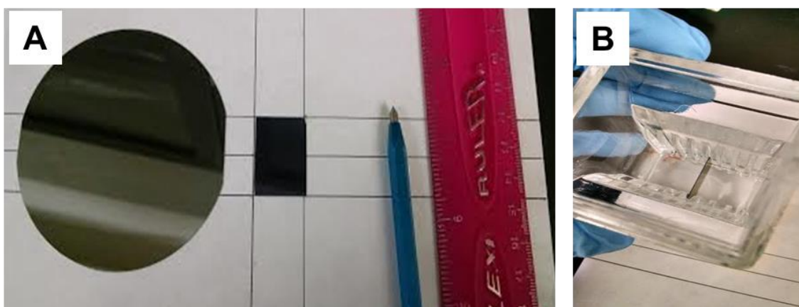
Figure D.1. (A) A silicon wafer and a score cut silicon wafer using a diamond scribe and a ruler. (B) Score cut silicon wafer placed in a staining jar to separate the wafers for cleaning in a base piranha solution.
