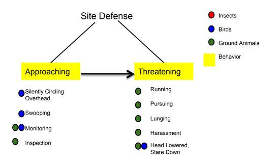
Figure 5.2: Final Site Defense tree for implementation in simulation on the AirRobot AR100B. Biological inspiration for the expression is reflected in the dots beside each expression with red for insects, blue for birds, and green for ground animals. Additionally, the highlighted words are for the names of the behavior represented by those expressions.
