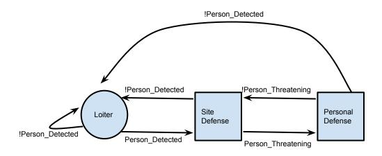
Figure 4.2: Basic escalation strategy FSA based on identified behaviors.
