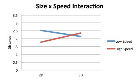
Figure 7.1: Interaction (p < 0.0001) of Speed with Dimensionality of the robots motion, where an increase in Dimensionality resulted in decreased distance in the low speed condition and increased distance in the high speed condition
