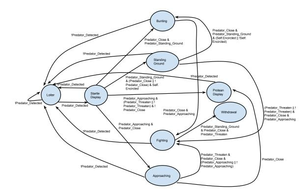
Figure 3.4: A finite state machine depicting the triggering of Personal Defense behaviors discovered through a review of literature.
