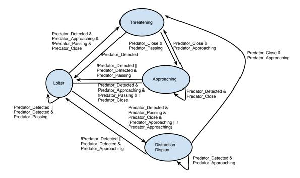
Figure 3.2: A finite state machine depicting the triggering of Site Defense behaviors discovered through a review of literature.
