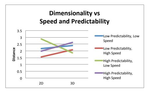
Figure 7.5: 3-way interaction (p < 0.008, p < 0.0001) with Dimensionality of the robots motion with both Speed and Predictability, where an increase in Dimensionality resulted in increased distance in all conditions except those robots with both high predictability and low speed.
