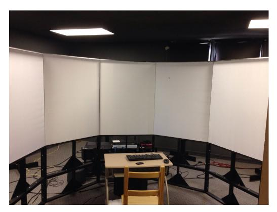
Figure 6.3: CAVE environment used in Study 1. Simulation projected on 5 screens (3600x1080) with participant interacting while seated at table.
