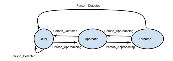
Figure 4.3: Site Defense escalation strategy for robots based on identified behaviors.
