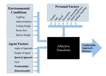
Figure 4.1: "Comfortable Distance" Model, incorporating the environmental conditions, agent factors, and personal factors identified from the literature. The transform black box represents the interactions between the factors, which can be partially gathered from the literature. The output is the distance that a human would feel comfortable being distanced from a robot or another human.
