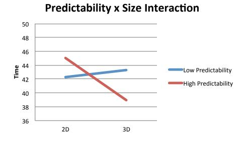
Figure 7.4: Interaction (p < 0.004) of Predictability with Dimensionality of the robots motion, where an increase in Dimensionality resulted in decreased time in the high predictability condition and increased time in the low predictability condition.
