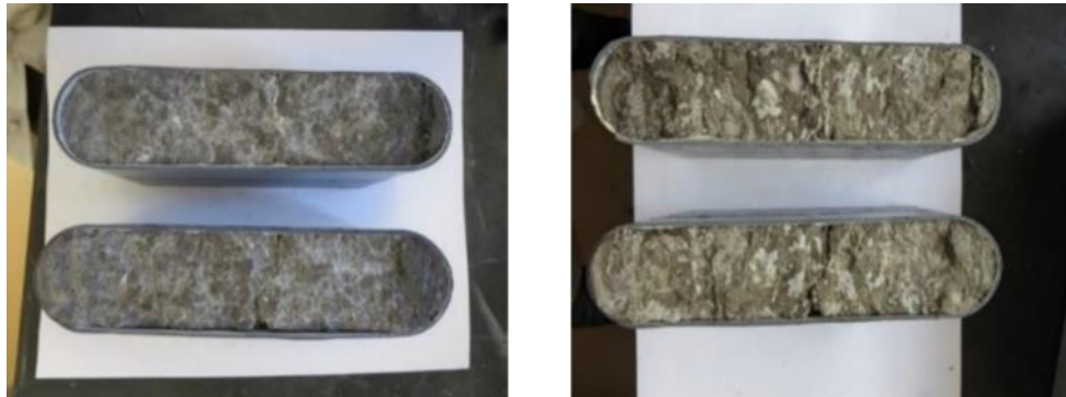
Figure 11. The image of core sample before (left) and after (right) acid etching test
