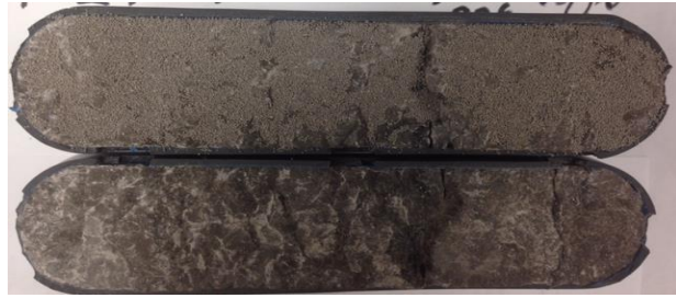
Figure 12. The image of prepared sample for propped conductivity test
