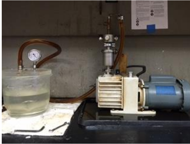
Figure 10. The image of water saturation apparatus
