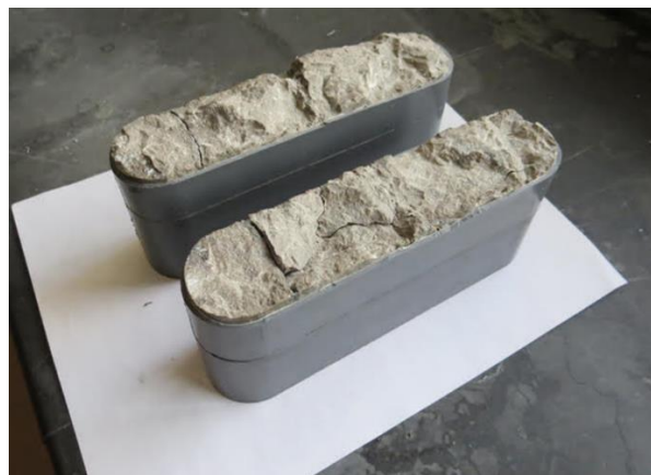
Figure 9. The image of prepared sample for acid etching test
