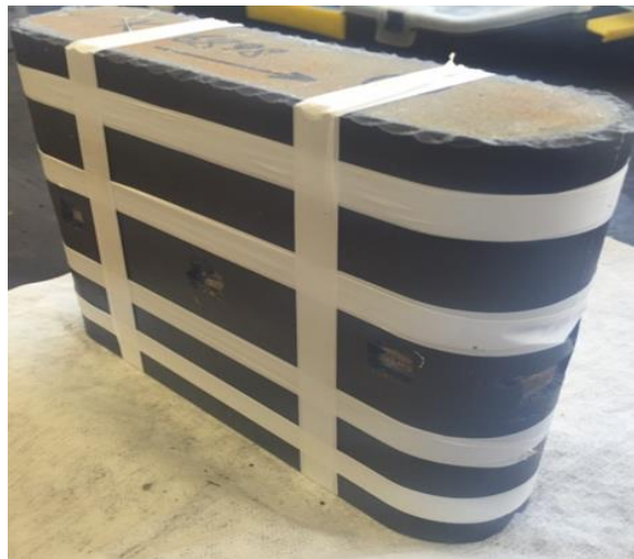
Figure 13. Prepared core sample for conductivity test
