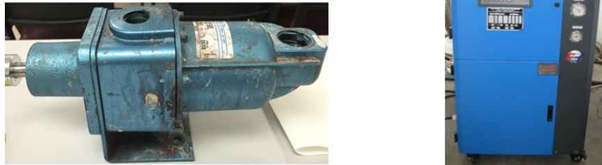
Fig. 14. Progressive cavity pump (left) and air-cooled water chiller (right)
