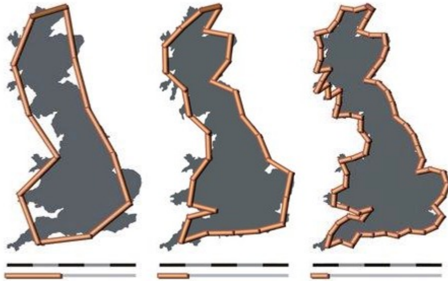
Figure 15. Measuring the length of a coastline using rulers of varying lengths.
