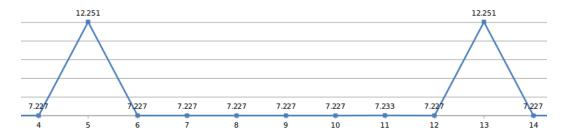
Figure B.1: Graph showing the timing results of sections being read with the extra 5 ms jump. X axis is section being read, Y axis is time in milliseconds.
