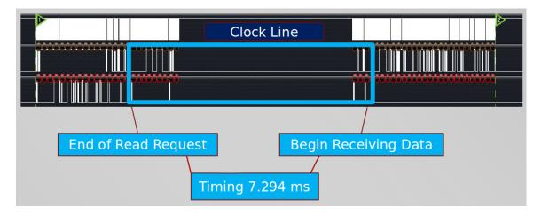
Figure 3.2: Reduced delay on tag time read, timing from logic analyzer.
