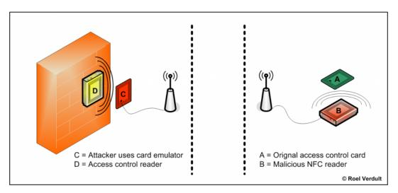
Figure 1.3: Relay attack example. Tag A and Reader D are authentic. C is the emulated tag (proxy) and B is the fake reader (mole). B and C are connected over some communication medium [33].
