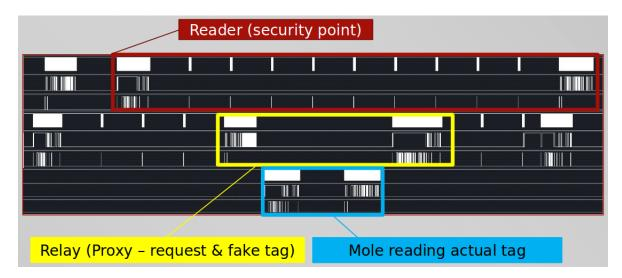
Figure 3.6: Timing analysis of relay attack using logic analyzer. Three different PN532 boards are pictured here, top: security point, middle: proxy on relay, bottom: mole on relay.
