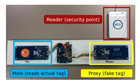
Figure 3.5: Arduino and two PN532 boards used to create our NFC relay system.
