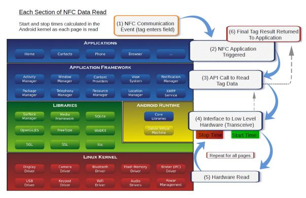
Figure 3.9: Android Architecture [44] with timing shown. Timing starts before HAL layer which sits between the kernel and library layer.
