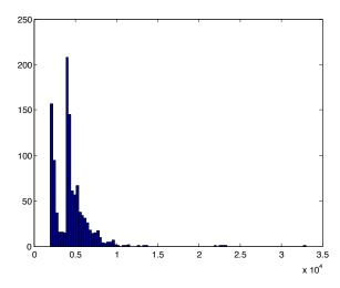
Figure 3.8: Histogram plot of tag read times in Android. The majority of reads are at about 4.5 ms or less. Y axis is sections read over 62 tags, X axis is time for read on each section.
