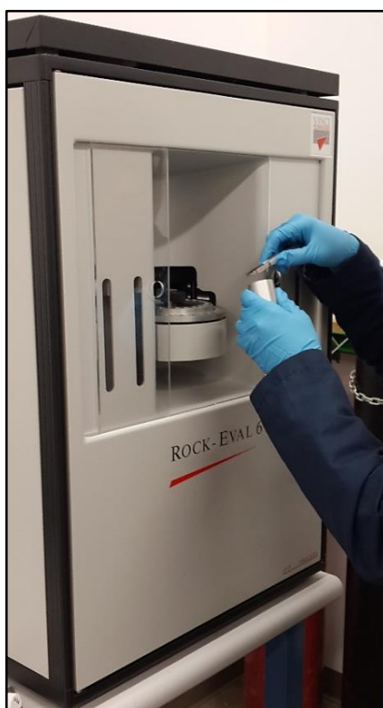
Figure 15: Rock-Eval 6 used for Rock-Eval pyrolysis located at W.D. Von Gonten Laboratories, College Station, Texas.
