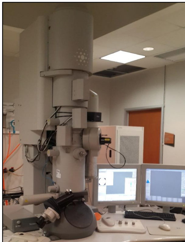
Figure 16: FEI Tecnai G2 F20 ST Microscope used for TEM images located at the Microscopy Imaging Center, Texas A&M University.
