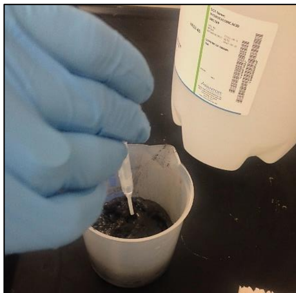
Figure 4: Adding HCl to sample in beaker. This step dissolves the carbonates that was present in the organic-rich mudrock sample.
