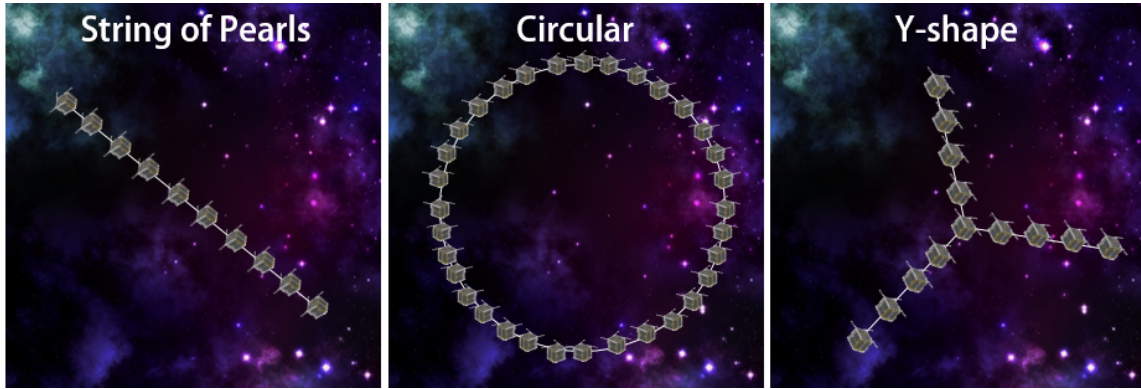
Figure 2.11: Various aperture formation geometries.
