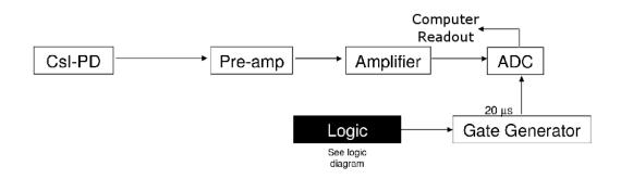
Figure 2.7: Electronics diagram for the CsI-PD signals of rings 12-15.
