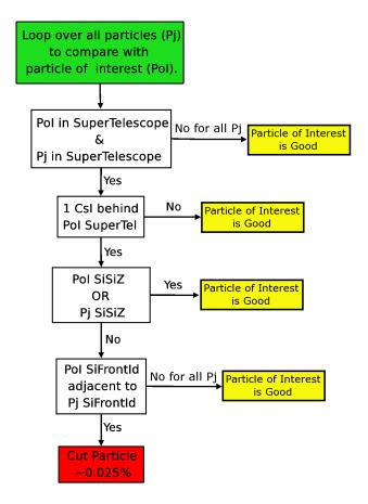
Figure 2.16: Flow chart depicting the process in which particles were compared in order to make sure that two particles were not identified in a supertelescope in which two silicon detectors were placed in front of 1 CsI.
