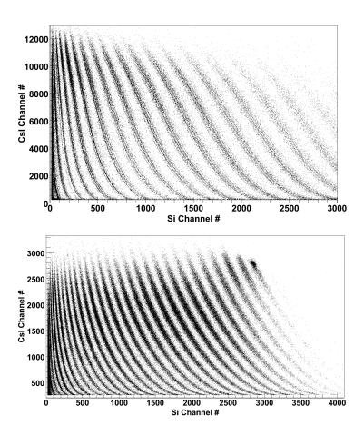
Figure 2.11: Silicon front-plane signal versus CsI signal (top) and silicon back-plane signal versus CsI signal (bottom).
