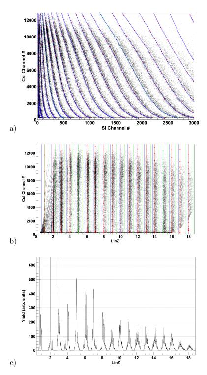
Figure 2.12: The linearization process is presented showing a 2-D Si-CsI plot (Panel a), the linearized 2-D plot (Panel b), and the 1-D projection (Panel c) of the linearization.
