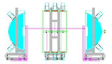
Figure 2.3: Side-view depiction of the TAMU Neutron Ball (without charged particle array). The three sections, consisting of two hemispheres and the center cylinder, are shown separated demonstrating the ability to move each section of the neutron ball independently.
