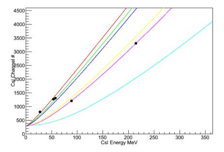
Figure 2.19: Example of CsI calibration showing the CsI slow signal channel versus the energy. The calibration points (black circles) were used to constrain the parameters of Equation 2.9. The energy calibration for protons (red line), deuterons (green line), tritons (blue line), <sup>3</sup>He (yellow line),  $\alpha$  (pink line), and <sup>7</sup>Li (light blue line) are shown.
