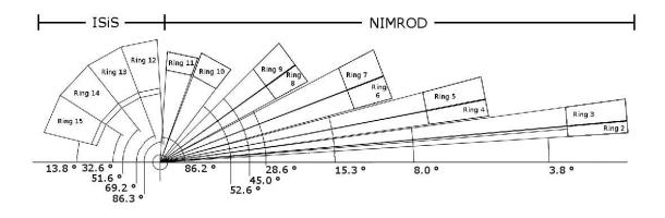
Figure 2.1: Side view of the charged particle detectors of the NIMROD-ISiS array. Each ring is labeled with the corresponding lab angle. The projectile beam is traveling from the left to the right in this figure.
