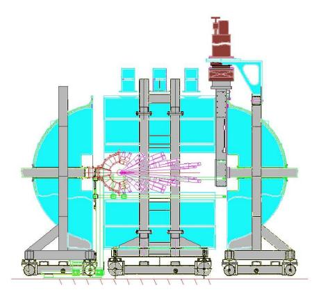
Figure 2.2: Schematic of the NIMROD-ISiS array showing the charged particle array housed inside the neutron ball. The projectile beam is traveling from the left to the right in this figure.
