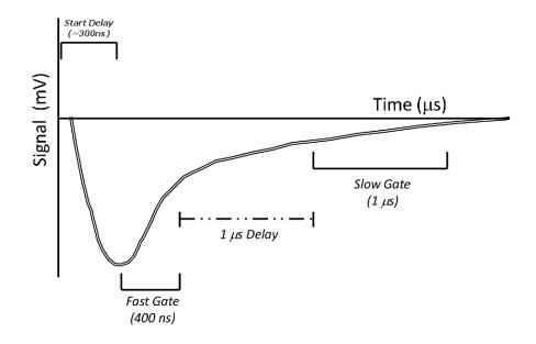
Figure 2.6: Illustration of the signal resulting from the CsI-PMT detector. Both the fast and slow signal gates are shown along with the 1  $\mu$ s delay and the start delay (300 ns).
