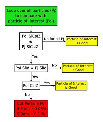
Figure 2.15: Flow chart depicting the process in which particles were compared in order to make sure that two particles were not identified in a detector module in which one silicon detector was placed in front of two CsI detectors.
