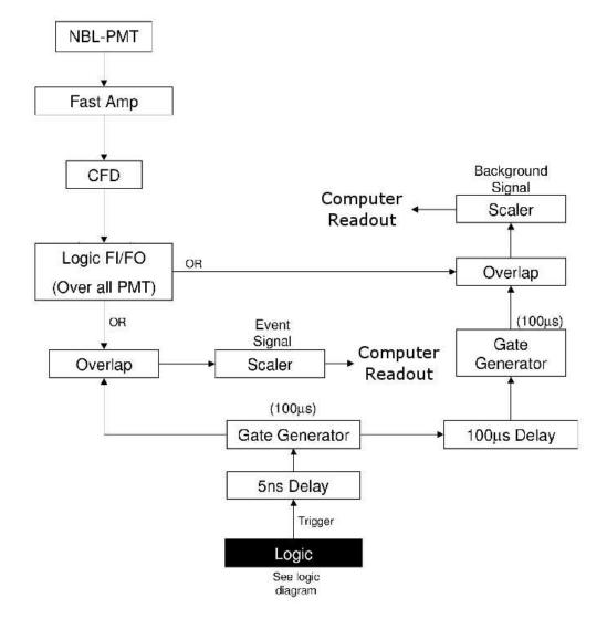
Figure 2.8: Electronics diagram for the PMT signals of the Neutron Ball.
