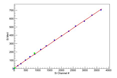
Figure 2.17: Example of a silicon calibration. The silicon energy from the punchthrough points is plotted as a function of the silicon signal channel number (blue circles). The fitted energy calibration, Equation 2.8, is shown as the black line. The calibration points from the 100 MeV  $\alpha$  and 500 MeV <sup>20</sup>Ne beams are shown as the green squares.
