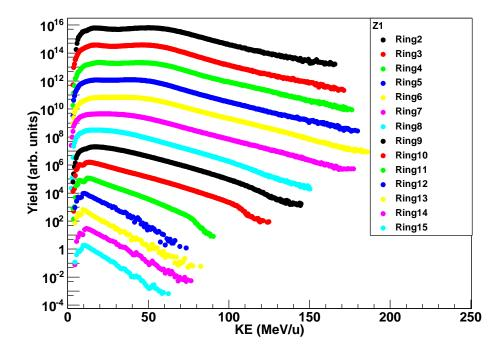
Figure 2.20: Energy spectra of the Z=1 fragments for each ring of the NIMROD-ISiS array for the 35 MeV/nucleon  $^{64}\rm{Ni}+^{64}\rm{Ni}$  system.
