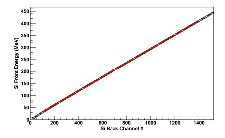
Figure 2.18: The energy determined from the front-plane silicon calibration is shown as a function of the silicon back-plane channel number (open circles). The calibration was determined by fitting Equation 2.8 (red dashed line) to the data.
