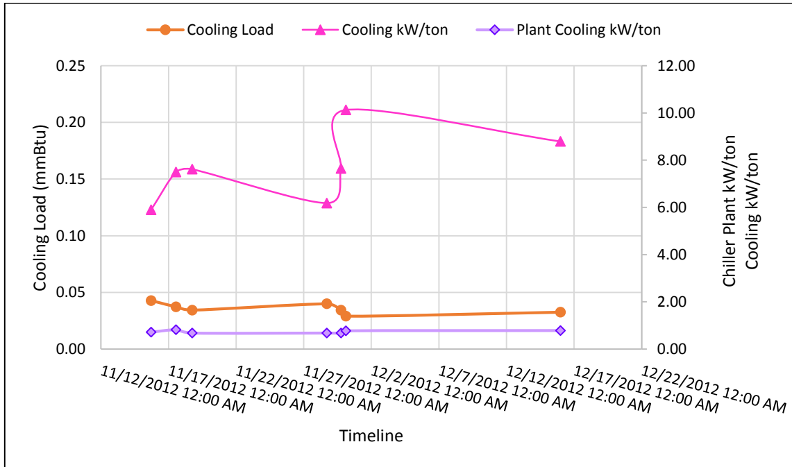
Figure 43 Cooling Load, Chiller Plant kW/ton and Cooling kW/ton from 11/15/2012-12/16/2012
