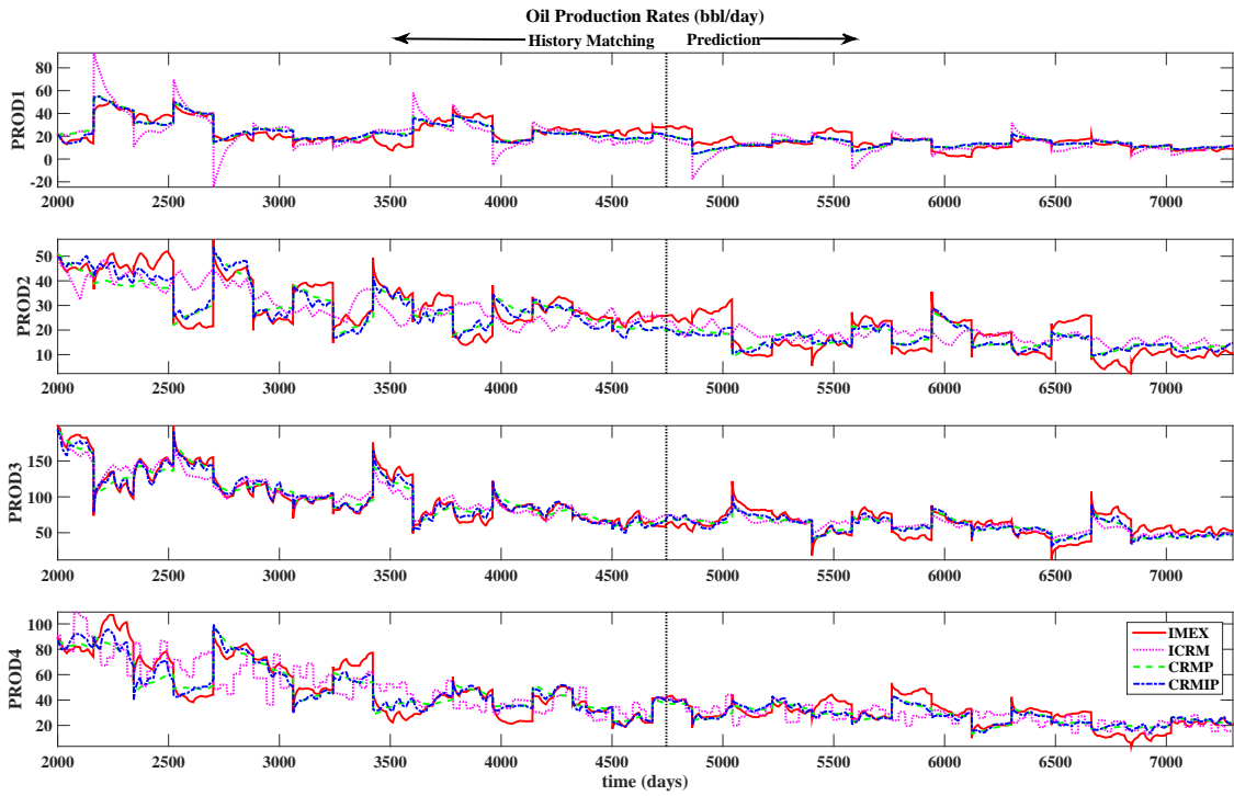
Figure C.10: Oil production rates (bbl/days) for ICRM, CRMP and CRMIP compared to the production history for producers 1 to 4 (case 3).
