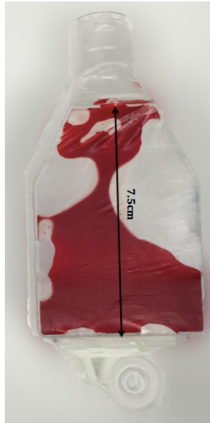
Figure 1. The blood-feeder device developed out of a 25 cm 2 cell culture flask (Corning Incorporated, NY) used to conduct the blood-feeding behavioral assay with Ae. aegypti . The device is wrapped in parafilm with 1mL of defibrinated rabbit blood pipetted in a gap formed between the culture flask and parafilm.
