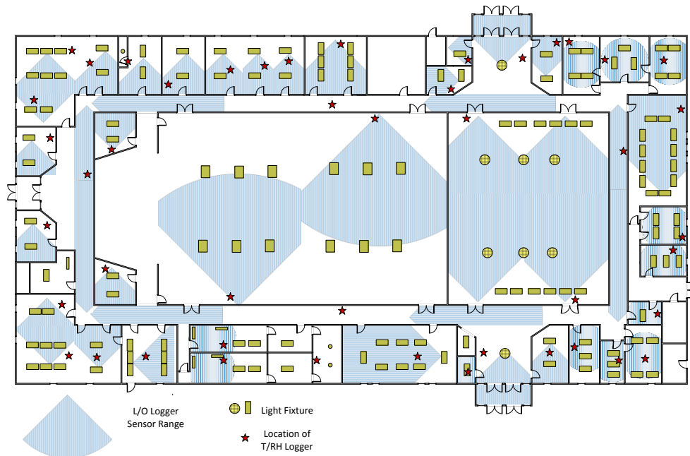
Figure 5. Placement of Light/Occupancy and Temperature/Relative Humidity data loggers in the church.
