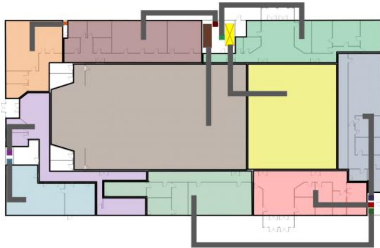
Figure 3. Zoning of the church buildings for the different HVAC systems.
