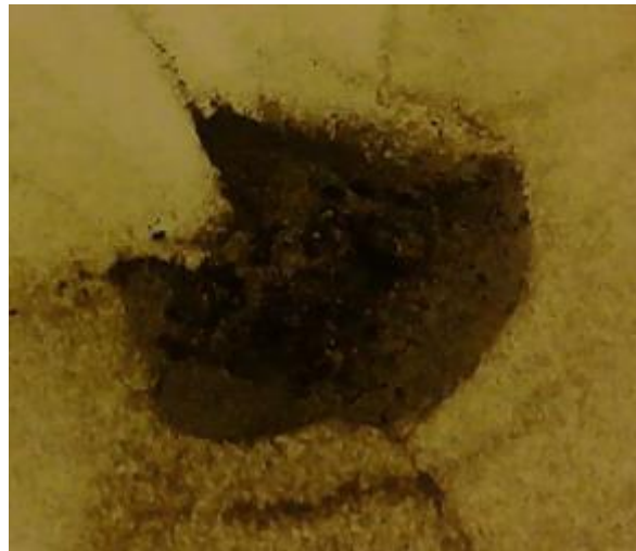
Figure 2.60 – Inner materials sample for liner #2 after the acid reaction
