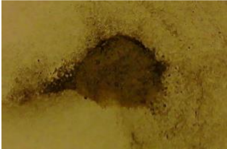
Figure 2.37 – Inner materials sample for the liner #2 after the acid reaction
