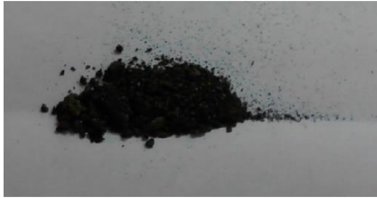
Figure 2.26 – Sample of the blocking materials taken from the outer surface of liner #2
