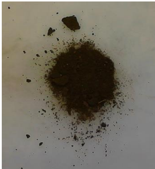
Figure 2.34 – Inner rust and scale sample of liner #2
