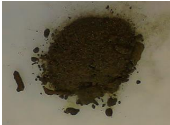
Figure 2.57 – Inner rust sample of liner #3
