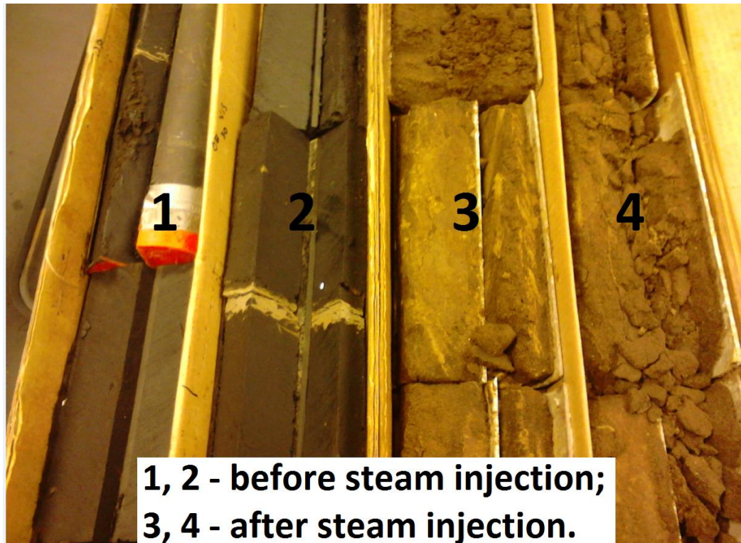
Figure 3.28 – Sandstone reservoir rock samples before and after steam injection
