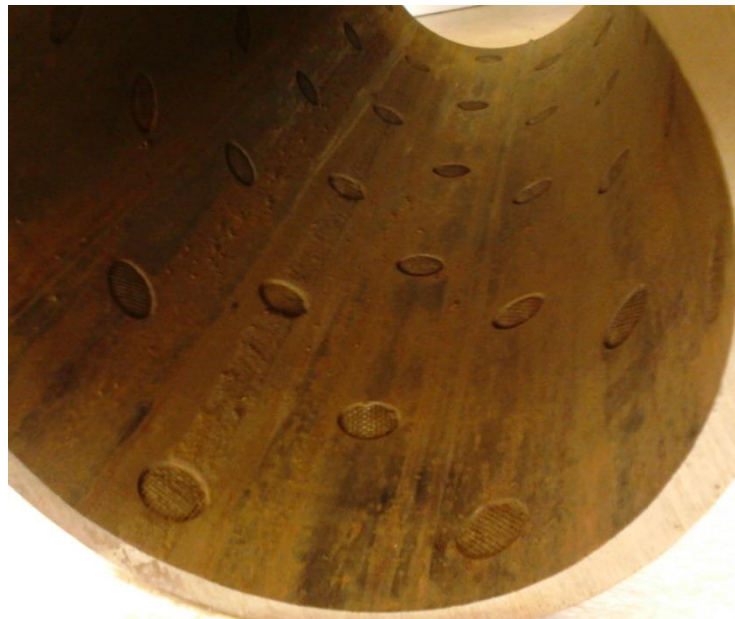
Figure 2.33 – Inner surface of liner #2
