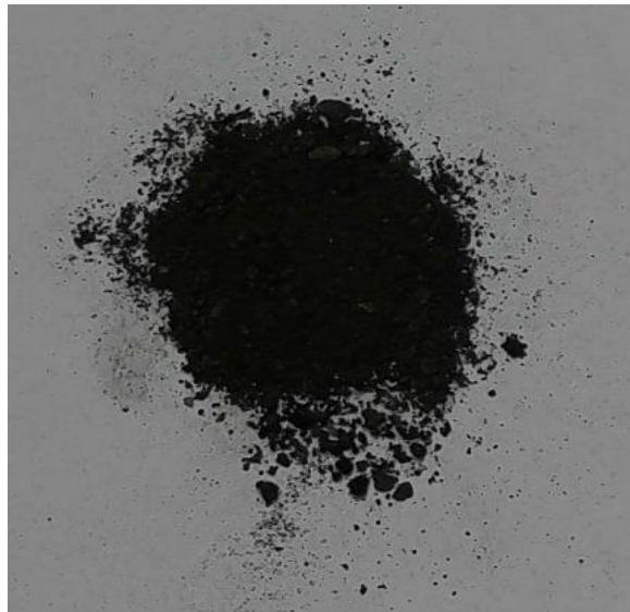
Figure 2.30 – Outer scale for the liner #2 after the acid reaction
