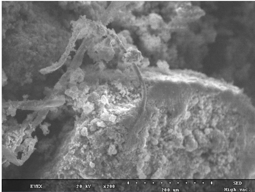
Figure 2.46 – Outer scale (bottom) electron microscope picture (magnification is 200)
