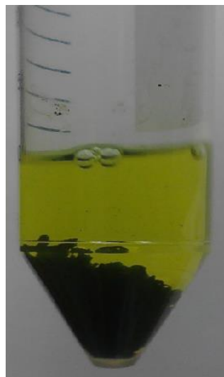
Figure 2.11 – Acid solubility test for outer scale from the bottom part of liner #1
