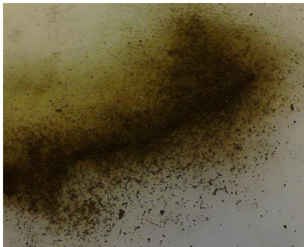
Figure 2.18 – Inner rust sample of liner #1
