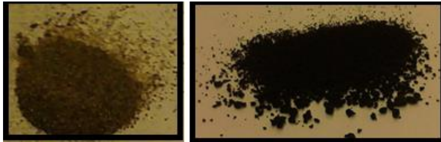
Figure 2.12 – Outer scale for liner #1 after acid reaction
