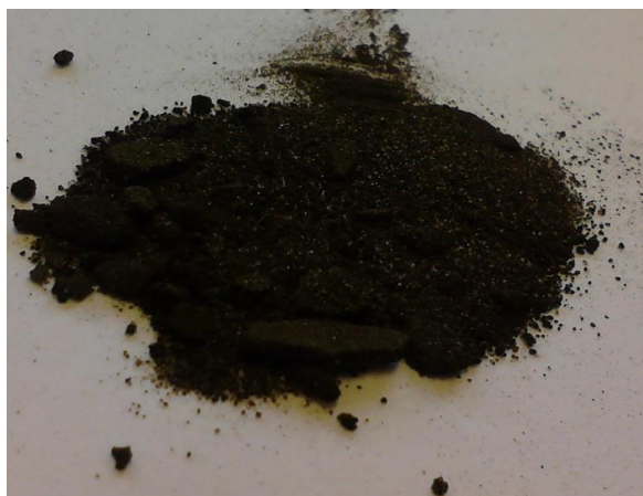
Figure 2.72 – Sample from the bottom part of liner #1 after the reaction with xylene
