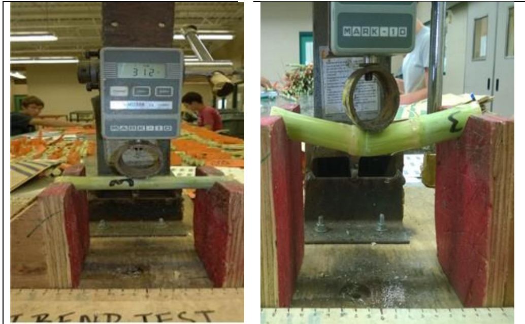
Figure 2. Two different loading configuration on a three-point bending device: (a) loading at individual internode, and (b) loading at the node.
