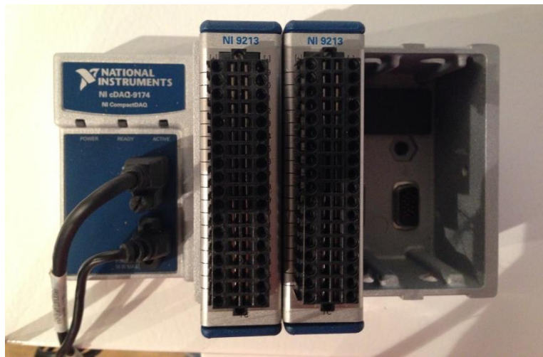
Figure 3. Photo of the NI thermocouple modules and compact DAQ for temperature measurements
